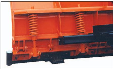
The recoil force of each compression spring can be adjusted on its threaded shaft for a precise adjustment to your specific plowing needs. This exclusive feature also allows for an easier and safer maintenance to the trip blade mechanism.
